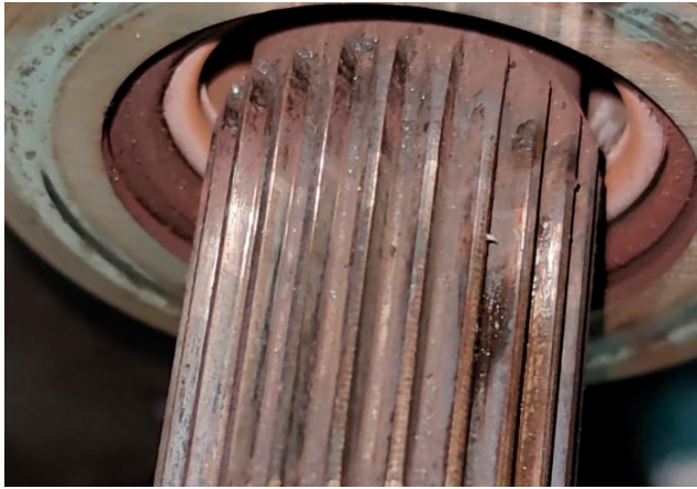
Image 3: Gearbox input shaft with increased spline wear
