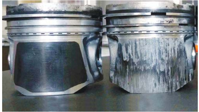
Surface 1 Surface 2 Piston skirt seizure on only one side
