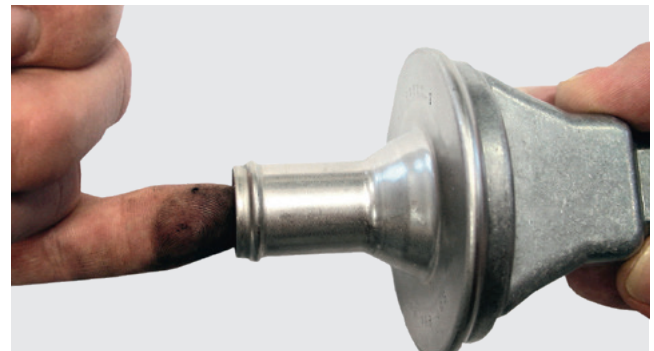
Fig. 1: Simple inspection of the non-return valve
