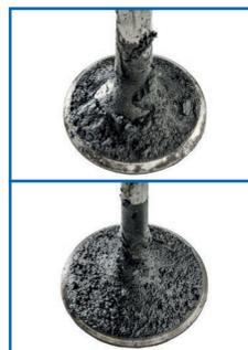
**Symptom:** Poor starting. Loss of power. Blue smoke from exhaust (when throttle closed).
