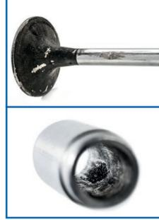
**Symptom:** Poor performance due to low compression. Mechanical breakage due to sticking valves.
