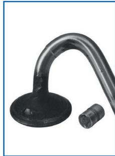
**Symptom:** Excessive mechanical noise, bent stem and possible head detachment.
