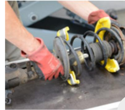
8. Ideally replace all rubber components and install these on the new shock absorber from Herth+Buss. Important: when mounting the spring cap on the suspension strut, ensure that the guide mount sits on top of the one on the shock absorber.
