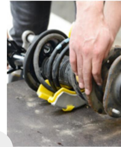
Tip: on older vehicles, it is also recommended to replace the top strut mounting at the same time, as this will avoid any additional work at a later point.
