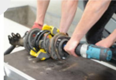
7. Remove the exposed shock absorber from the spring.
