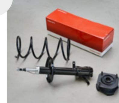
10. The assembled suspension strut with the replaced shock absorber can now be installed on the stub axle again. The same applies for the previously removed sensor system and brake line.
