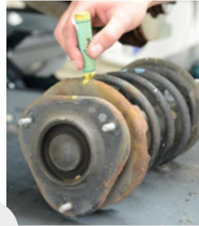
6. In the next step, compress the suspension strut using a spring compressor. Once the spring is sufficiently compressed, the nut can be loosened from the top strut mounting, and the top strut mounting can be removed together with the spring cap.
