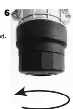
Tighten the cap using 25± 5Nm of torque.
