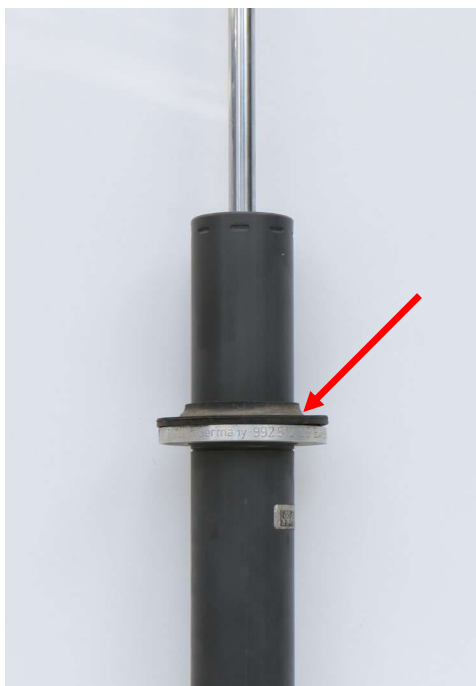
Abb. 5: Federteller demontieren Fig. 5: Dismantle the spring plate
