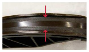
Excessive wear on plastic part of the guide. Inadequate lubrication has caused the chain to elongate and collide with with the guides.
