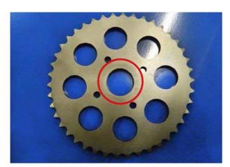
Fig. 1 Sprocket without key slot
