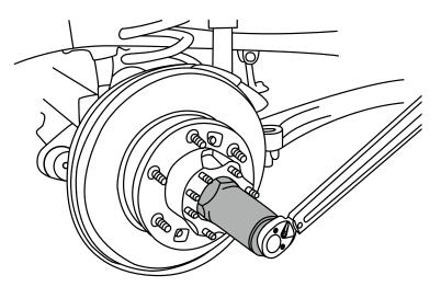
Failure to use the correct tools and adhere to the correct instructions could result in incorrectly adjusted wheel bearings which in turn could result in premature bearing failure.
