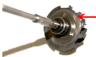
Abrased back panel on turbine wheel - causes noises
