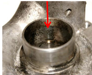
Oil mist in compressor housing
