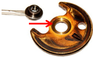
Tinted thrust washer due to axial thrust
