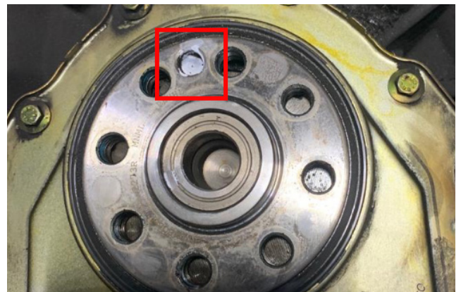
Figure 2: Reference mark on the crankshaft
