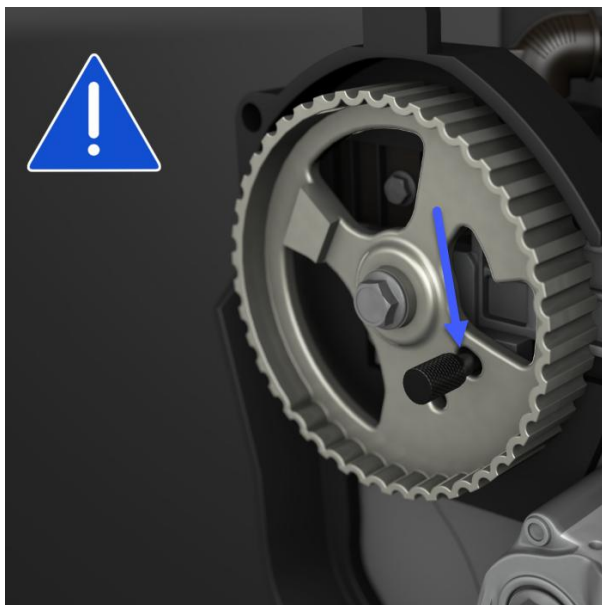
Camshaft and camshaft sprocket locked Slotted hole in 4 o'clock position
