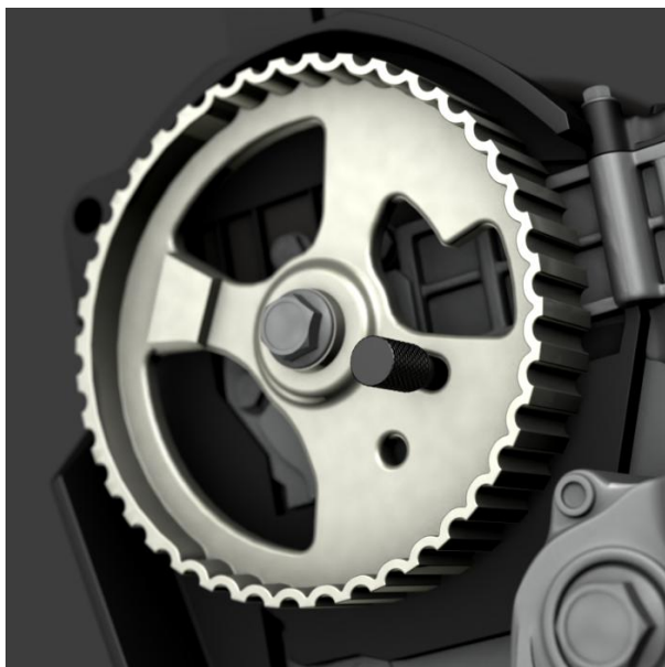
Timing belt / TDC: Slotted hole in 4 o'clock position
