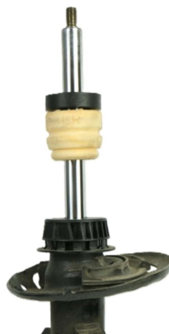
Fig. 1: Bump rubber and rubber spacer
