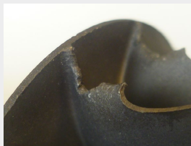
Damaged exhaust turbine
