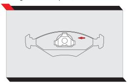
points in the same direction as the wheels turn during forward driving.
