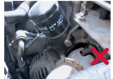
Figure 3: When topping up the engine oil or changing the oil filter, the alternator may need to be protected
