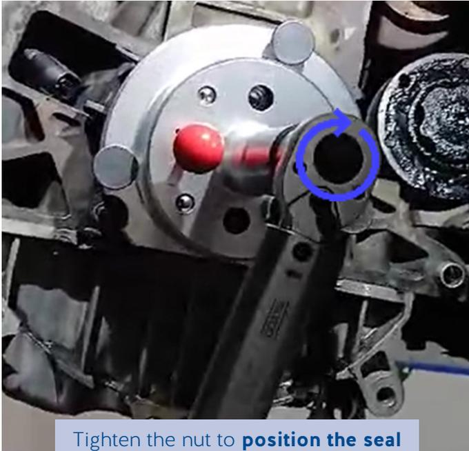
Tighten the nut to **position the seal** in its housing
