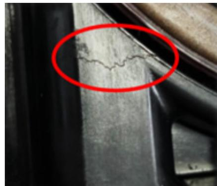
Cracked oil seal during assembly due to not using the special tool.
