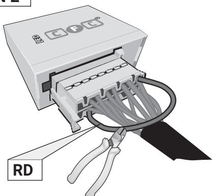
Pin 11 and Pin 2 disconnected
