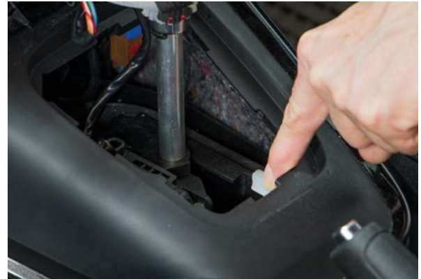
The shift lever can be unlocked using a push button
