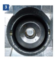
Make sure that the position of the retention pins is correct when the upper lip ascends, so the set will be well positioned.
