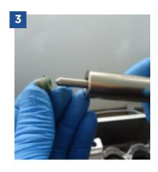
➤ Introduce the new valve seal. Make sure the housing is totally clean and hit the base of the tool until it is completely fixed.
