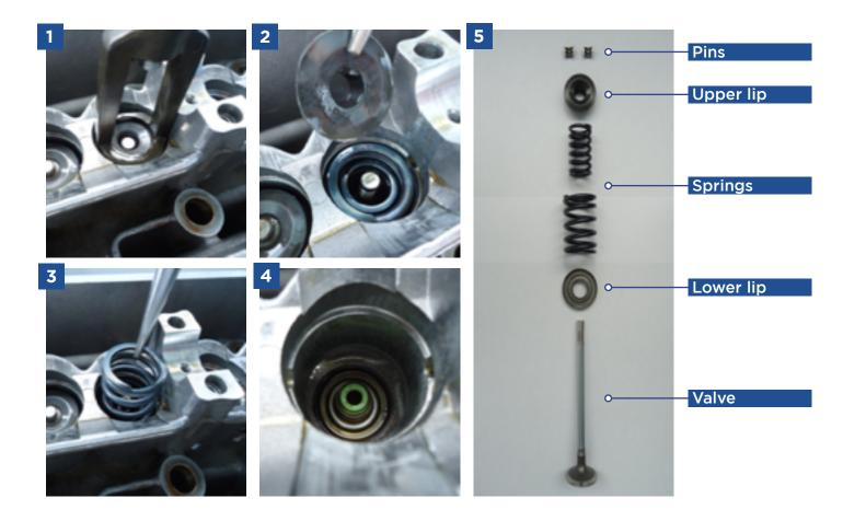
> Place the remover taking the stem seal from the metal body and remove from its housing, hitting the seal with the tool to remove it from the head.
