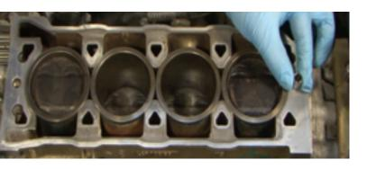
Do not turn the crankshaft once you you remove the tools to pin up liners.
