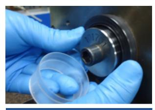
Assembly of the PTFE seal in its housing
