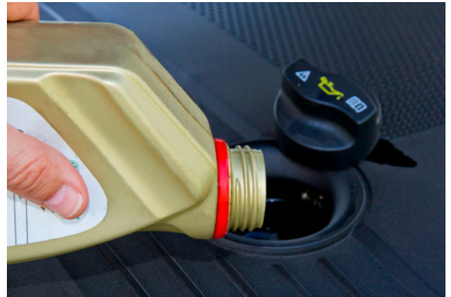
Figure 1: Unsuitable engine oil will cause premature failure of the timing belt
