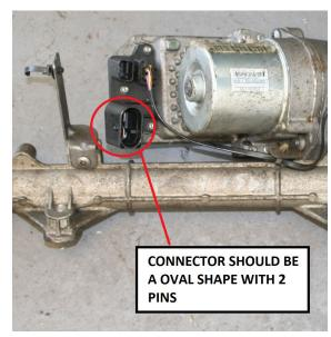
ERRM2004 has a Round shape connector each with a pin
