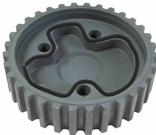
Ajusil silicone sealant at the back of the injector pump pulley
