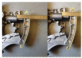
TEST METHOD: checking the position and distance after removing the locking key to check whether the piston brings the guide rail into correct position after mounting it and removing the key lock
