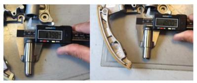
RESULT: The space between for OE is 0,07 mm and VAICO is 0,03 mm so that lower oil pressure on the VAICO piston cannot be the reason for too less tension. All returned samples show the same measures
