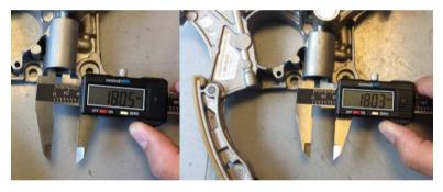
TEST METHOD: comparing diameter of bolt and bore to genuine to check the space between
