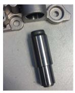
TEST METHOD: we removed the pistons from the tensioners and checked the pressure of the inner spring.
