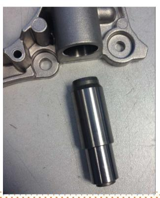
TEST METHOD: moving the piston inside the housing and removing it to check for scratches and damages
