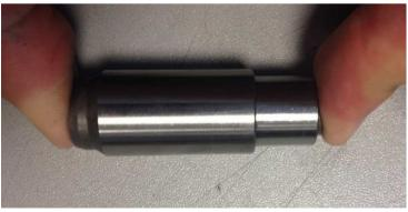
RESULT: OE and VAICO have the same pressure and will provide the same inital tension on guide rail and chain . All returned samples show perfect performance for the spring and its initial tension
