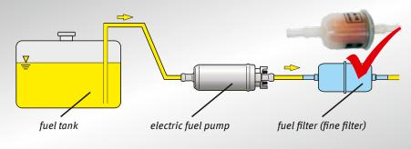
A fuel filter must always be installed on the thrust side of the fuel pump.
