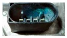
Built-in plug with traces of corrosion
