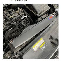
5 Unscrew coolant pipe from intake manifold and set it aside so that it does not obstruct
