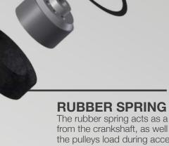
The rubber spring acts as a damper to absorb torsional energy from the crankshaft, as well as functioning as a spring to control the pulleys load during acceleration and deceleration.
