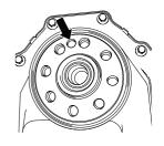
As opposed to a conventional dowel pin, these DMFs are timed via a hole in the DMF (Picture 1) and an indent in the crank shaft (Picture 2).
