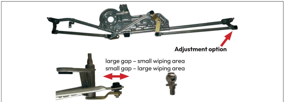
Before installing the wiper linkage, the wiper motor must be moved to the zero position. The size of the wiper field can be adjusted by rotating the eccentric bolt, preventing the wipers from hitting any obstacles.
