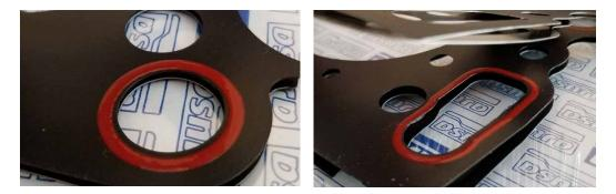
We also find **reinforcements in other areas** as the bridge between cylinders, the timing chain, etc.
