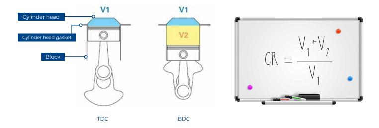
The **cylinder head gasket** is **part of V1**, so if we modified its thickness, we are changing the CR.If we decrease its thickness, we are increasing its CR and otherwise, if we increase its thickness, we are decreasing the CR.
