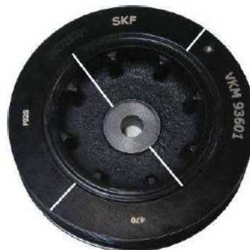
Worn Damper! Needs to be replaced!
