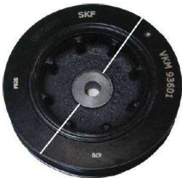
Damper in good condition
