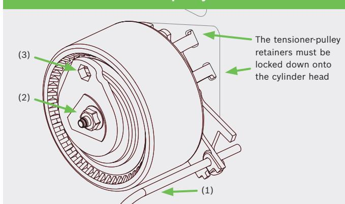
Fit the timing belt as specified by ESI[tronic]-M and remove the fixing (1) and locking pins of the tensioner pulley.
