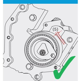
Then, turn the crankshaft clockwise six full rotations. Lock the flywheel using the locking pin (tool Mot.582-01). Slightly move the crankshaft back and forth to make sure the locking pin has been placed correctly. The marks need to be aligned. Remove the locking pin.
