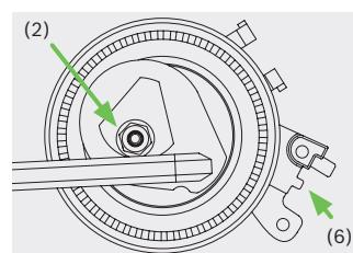
Turn the tensioner pulley clockwise until the needle reaches its central position (6). Tighten the tensioner-pulley nut (2) to 24 Nm.
