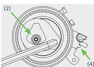
Turn the tensioner pulley counterclockwise until the needle points at maximum timing-belt tension (4). Tighten the tensioner-pulley nut (2) to 24 Nm.
