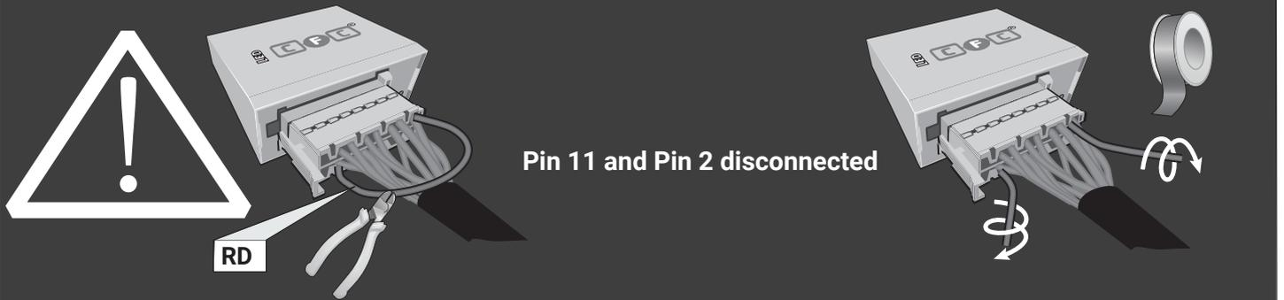
Pin 11 and Pin 2 disconnected
