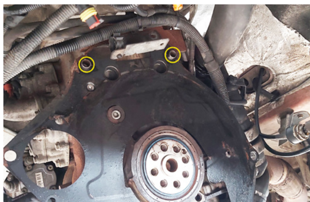
Image 1: The alignment dowels on the cylinder block
