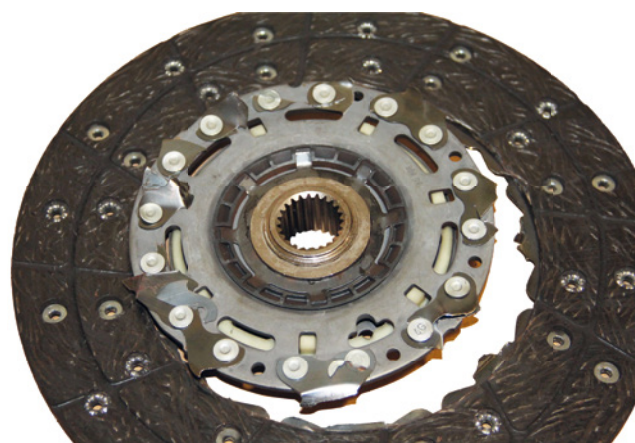
Image 2: Broken clutch disc hub
