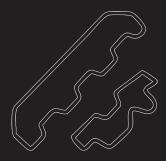
Plastic guide crumbles or break, sending debries into sump and clog the pickup strainer.
