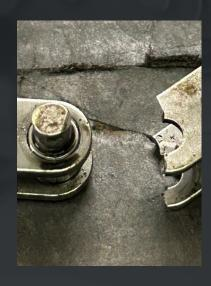
Heavy carbon build up and debris on returned parts. This is caused by many factors from age to malfunctioning breather systems and EGR. Long service intervals allows carbon to build up within the engine which can be accelerated by many other factors. Carbon build up is the number 1 cause of replacement chain failure
