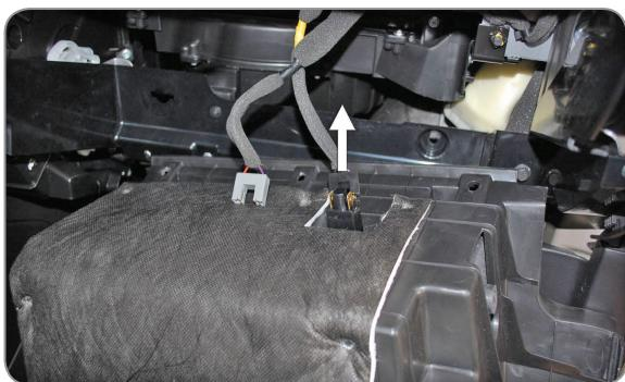
EN Disconnect the electric circuit
