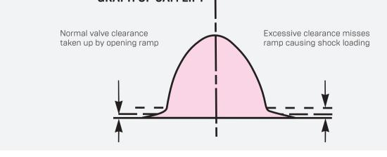
• The valve seat must be concentric with the valve guide. Any eccentricity that exists between the valve seat and guide will force the valve sideways. • Excessive valve guide wear will occur as a result of this which can lead to a fatigue failure of the valve stem.
