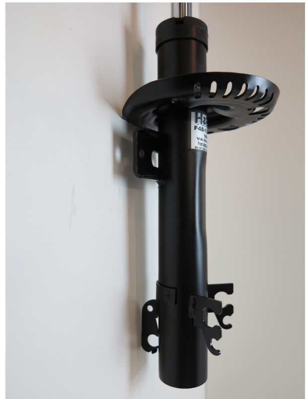
Pic 2: FA strut with welded sheet metal brackets
