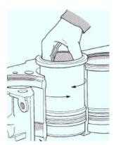
3. Using a dial gauge, **measure the height** between the cylinder liner projection and the block at the 2 points indicated. Always on the camshaft side.
