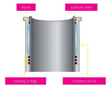
This system makes it necessary to seal the wet cylinder liner between these liners and the engine block, since there is coolant flow between both parts.
