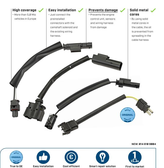
MEYLE no.: 014 810 9001, 014 810 9002, 014 810 9003, 014 810 9004 Applications: Mercedes-Benz engines M111, M271, M272, M273, M276, M274, M264, M282 (e.g. A, B, C, CLK, CLS, E-class and Sprinter)
