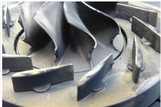
destroyed turbine wheel and VTG unit
