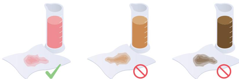
Flush the power steering system by removing the power steering lines from the steering rack. Take note of the oil condition – is it clean or contaminated? Contamination can be a sign of degradation in the power steering lines. The lines are often degraded internally, and thus can be difficult to spot – they are however often degraded simultaneously. If the system is not flushed, warranty will be voided.
