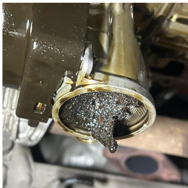
Oil pump clogged due to timing belt abrasion.
