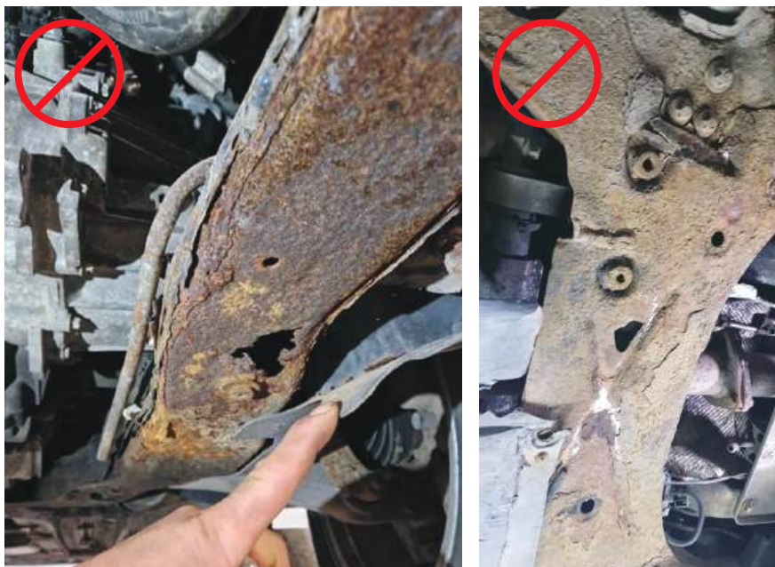
Structural damage of axle beams caused by corrosion.
