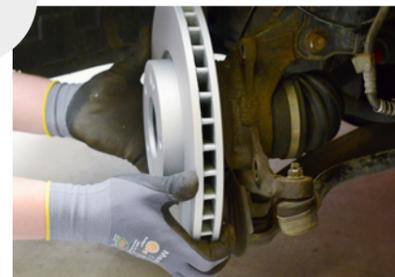
6. Now mount the new, perfectly fitting Herth+Buss brake disc onto the wheel hub. The new brake disc must be completely free of grease to ensure that the braking power is not compromised later on. Please note: it is not necessary to clean the brake disc or remove the coating before installation! After performing the repair, the vehicle should be braked hard four to five times from around 50 - 60 km/h during a test drive to remove the coating from the brake discs.
