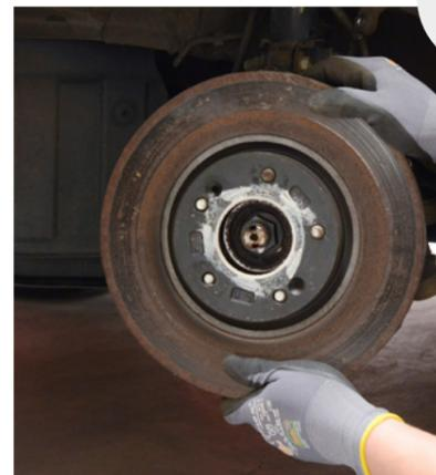
4. Remove the brake disc and check the brake components for damage, replacing them if necessary.
