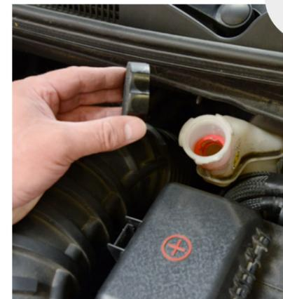
8. Before resetting the brake pistons with a suitable reset tool in the next step, you should first check the brake fluid level and extract a little of the fluid if necessary. Please be sure to observe the manufacturer's instructions when resetting the pistons!
