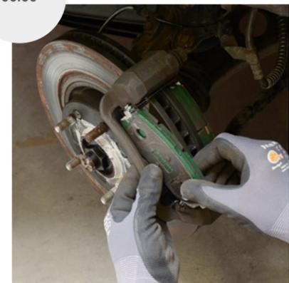
2. Release the brake calliper and remove the brake pads. Attention: when replacing brake discs, always replace the brake pads with them and replace all brake discs/ brake pads on the respective axle!
