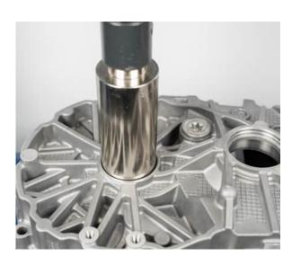
• Press the new ball bearing of the input shaft into the transmission housing
