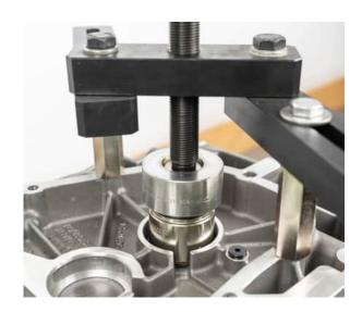
• Press in the new engine-side bearing outer ring of the output shaft **without** adjusting washer
