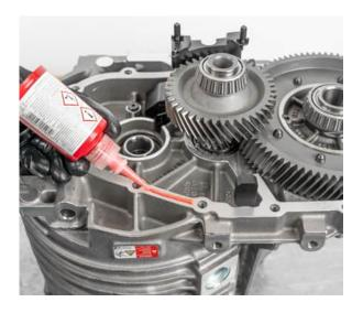
• Insert the screws and tighten to 20 Nm + 45°
