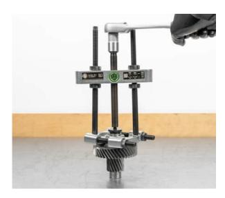
• Press the new transmission-side taper roller bearing onto the output shaft
