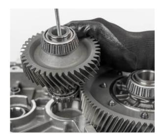
• Take the differential gear out of the engine housing
