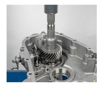
• Insert the differential gear and the output Oshaft into the engine housing
