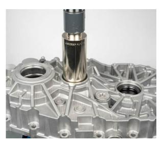
• Remove the transmission-side shaft seal of the differential gear
