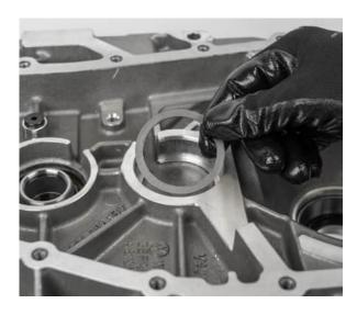
• Press the new engine-side outer bearing ring for the output shaft back into place
