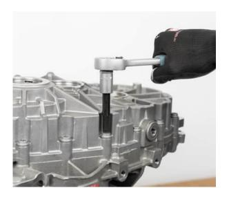
• Lift the transmission housing evenly up and off using a suitable tool (e.g. mounting lever)
