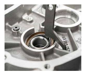
• Press in the new shaft seal of the rotor shaft to the previous installation depth
