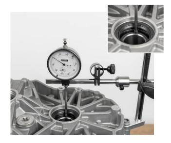
With your hand, press the differential gear upward on the opposite side so that it is up against the stopper and read the measured value
