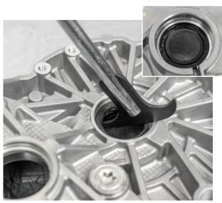
• Remove the transmission-side bearing outer ring using a suitable internal extractor
