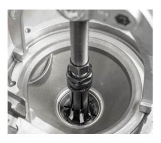
• Insert the previously determined adjusting washer (e.g. 0.90 mm) into the bearing seat
