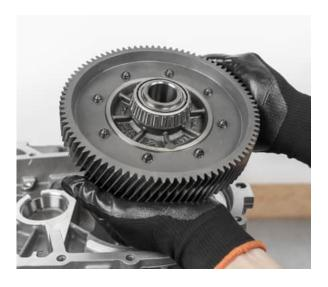
• Remove the engine-side outer ring of the output shaft again
