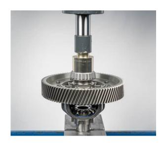
• Press the new engine-side taper roller bearing onto the differential gear
