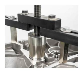
• Remove the engine-side outer ring of the differential gear
