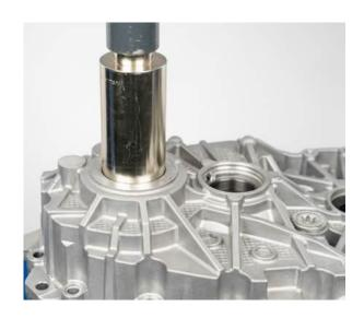
• Press the bearing outer ring of the output shaft out of the transmission housing
