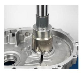
• Press in the new transmission-side shaft seal of the differential gear to the previous installation depth
