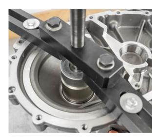
Press in the new engine-side shaft seal of the differential gear to the previous installation depth
