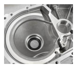
• Press in the new engine-side bearing outer ring of the differential gear **without** adjusting washer
