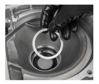
• Press in the new engine-side bearing outer ring of the differential gear
