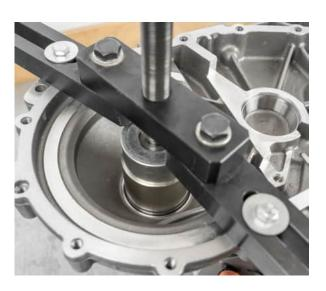
Remove the engine-side taper roller bearing of the differential gear
