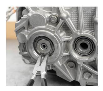
• Remove the snap ring from the output shaft
