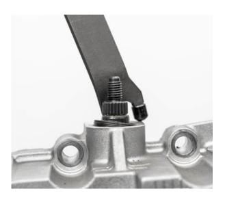
• Mount the new shaft seal to the previous installation depth using a suitable sleeve.
