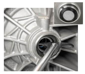
• Remove both sealing covers using a suitable tool e.g. Gedore Automotive KL-0369-59
