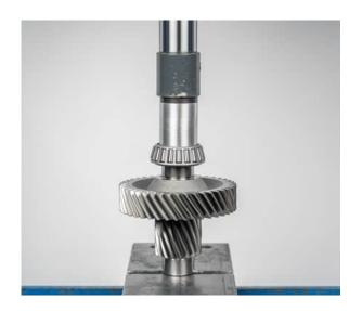
• Press the new engine-side taper roller bearing onto the output shaft
