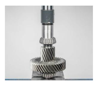
• Insert the differential gear into the housing
