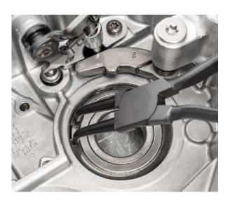
• Press the ball bearing of the input shaft out of the transmission housing
