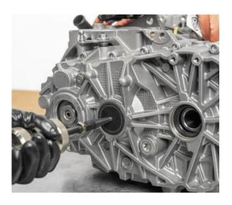
• Remove the snap ring from the input shaft
