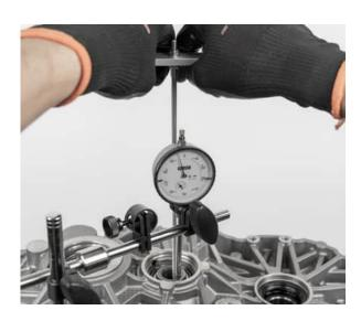
The required bearing preload is **0.25 to 0.30 mm**
