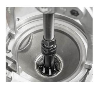
• Remove the baffle plate
