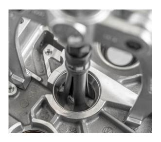
• Insert the previously determined adjusting washer (e.g. 1.20 mm) into the bearing seat
