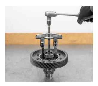
• Press the new transmission-side taper roller bearing onto the differential gear
