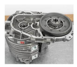
To be able to measure the axial clearance of the output shaft, a suitable lifting device, such as a threaded rod with a welded-on washer, is required
