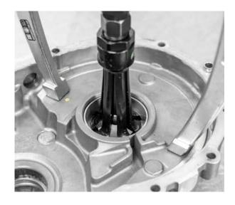
• Remove the baffle plate
