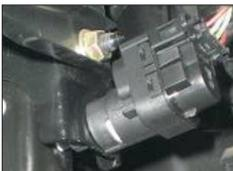
Insert the switch into the opening in the pedal assembly (there is only one possible position) and turn it approximately 45 degrees to the right to reach the final installation position. Turn without using force. If necessary, apply minimal pressure to the tappet.
