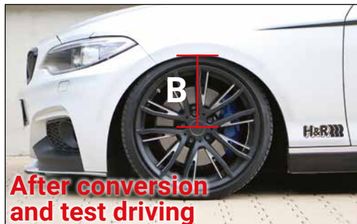
Measurement B: Wheel hub centre – fender edge
